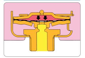
As the condensate temperature approaches steam temperature, the capsule fill boils and evaporates, increasing the internal pressure which expands the diaphragm.
