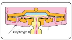
Even in an extreme case, where the valve plug is severed completely from the lower diaphragm, the condensate can drain through the hole in the valve plug center.
