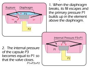
The closed valve causes condensate to accumulate.
